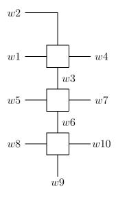
Executing the network with symbolic values confirms that the first component of the result is the minimum of the 4 input values:
