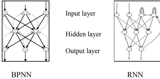
Figure 3 Architecture of BPNN and RNN
