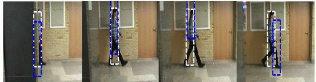
Fig. 2: A comparison of tracking accuracy between M 3 F-GWL(white) and M 3 F-PF(blue). M 3 F-GWL shows more accuracy in tracking a person when it becomes visible after occlusion in comparison to M 3 F-PF.
