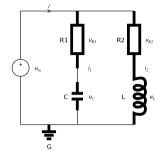
connect acp, r1p, r2pconnect r1n, cpconnect r2n, lpconnect acn, cn, ln, gpi = r1p.i + r2p.i
