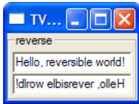
Figure 2. A Tangible Value and the GUI generated based on its type, with text boxes being used to interact with Strings.
