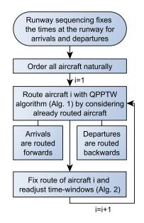
Fig. 3 Flow chart of general concept of the approach
