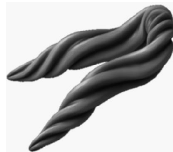
Figure 11: Reconstruction of a hairpin vortex tube, with grooves indicating velocity 2 .
