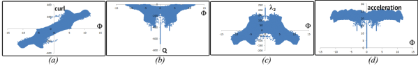
Figure 3: The scatter plot between the \Phi field and curl (a), Q (b) and \lambda_2 (c) and acceleration field (d), respectively, for the Double Gyre flow.
