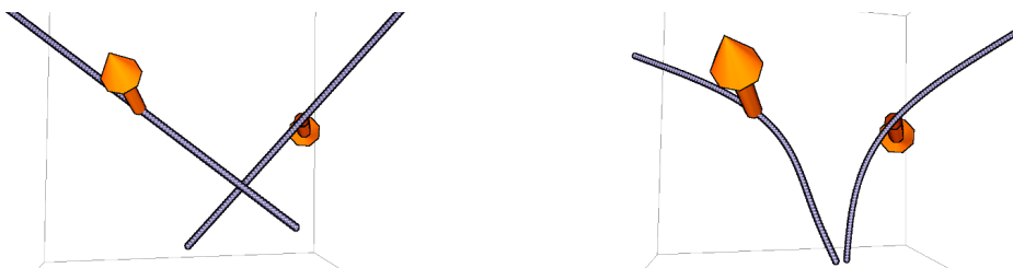
Figure 4.9: These illustrations demonstrate straight seeding curves vs integrated seeding curves. The representative vectors and locations are visualised with arrow glyphs. The left image shows the seeding curves crossing each other when aligned with the curvature vector. The right image shows the seeding curves following the curvature, not crossing, and remain orthogonal to the flow.
