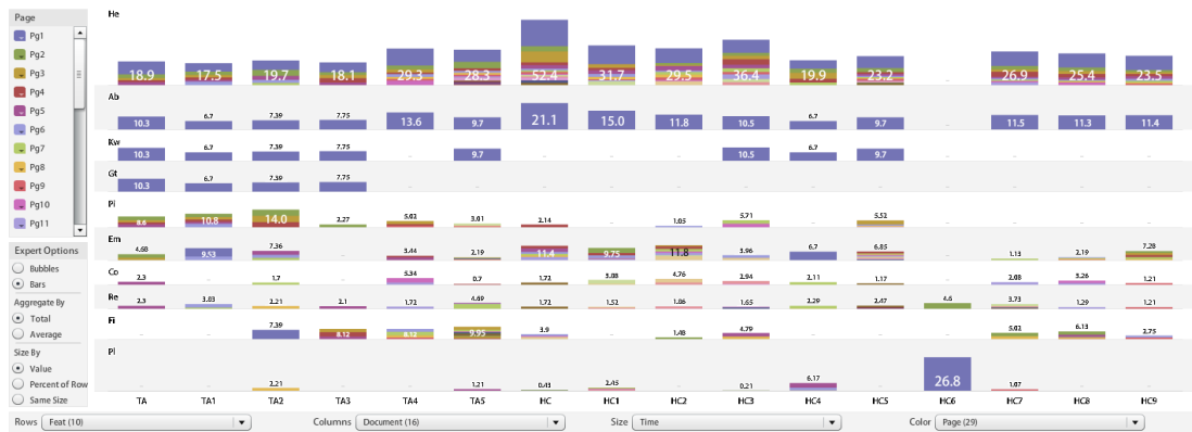
Figure 2.6: This figure shows a matrix chart in ManyEyes [VWvH + 07]. Rows are mapped to the document features, columns to the documents, colors to page number and size of each bar to time. Rows, columns and colors can only accept categorical data. This visualization depicts four variates at a time and displays the general view among the four variates.
