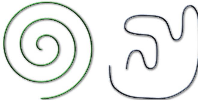
Figure 6.3: Both of these curves exhibit very similar curvature magnitude values. Therefore, a single global measure fails to distinguish streamline sufficiently. In this case, the tortuosity attribute would fair better but there are cases where this would also fail. A better method creates a distinctive signature for the streamlines using frequency-based attributes.
