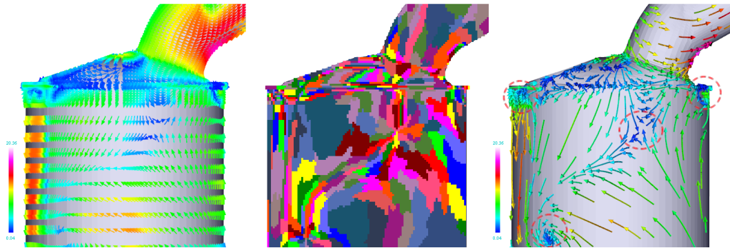
Figure 6.21: A screen shot of the visual result comparison between the direct flow visualization (left) and the feature-based visualization (right). (left) The cluttered direct flow visualization can't do a good job of extracting important flow features. (middle) Vector field clusters are generated and coloured in different colours. (right) Based on the generated clusters, shaded streamlets with arrow head are applied to reveal some flow features such as vortices and saddle points which are highlighted by red circles.
