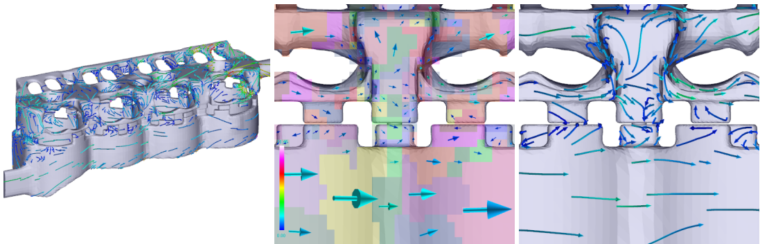
Figure 4.15: Various visualization options applied to depict vector field clusters on the cooling jacket surface - a composite of 228k unstructured, adaptive-resolution polygons: (left) the glyph visualization illustrating an overview of the flow field on the surface using \epsilon = 25\% , (middle) the glyph visualization and (right) the cluster-based streamlet visualization providing a close-up view on the area deemed interesting with \epsilon = 38\% and \epsilon = 35\% .
