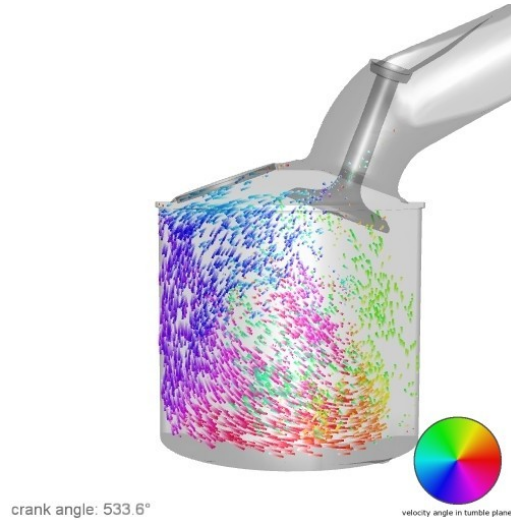
Figure 6: Pathlets visualizing tumble motion of flow. Image courtesy of Garth et al. [5]
