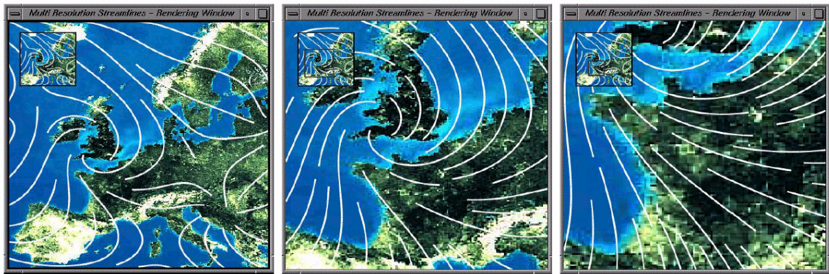
Figure 4: three images from an interactive exploration of a vector field using the MR viewer, image courtesy of Jobard and Lefer 62 . A suitable level of resolution can be chosen while maintaining a roughly constant stream line density.
