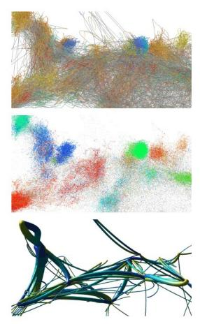
Figure 7: Abstraction of the pathlines. The upper figure shows all pathlines. The middle figure shows the vertices of all pathlines, coloured based on the detected clusters of slower motion. Positions of conserved water correspond to the larger clusters. The lower figure shows the extracted principal paths.
