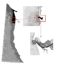
Figure 2: The CORIE computational domain extends along the continental shelf from British Columbia to California. An horizontally unstructured grid enables enhanced refinement in areas of primary interest, including the near-field plume, the estuary entrance and the navigation channel.
