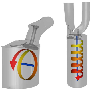
Fig. 13. Idealized in-cylinder flow through a gas engine (left) and a diesel engine (right). Figures 14 and 2 show our visualization of CFD data simulating such flows.
