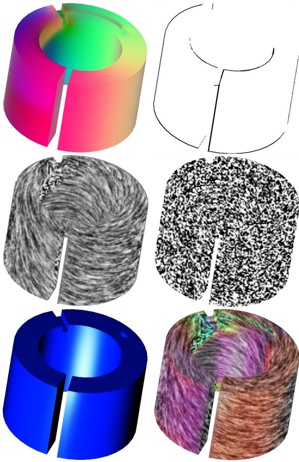
Figure 5: The 5 component images, plus a 6 th composite image, used for the visualization of surface flow on a ring: (top, left) the velocity image, (top, right) the geometric edge boundaries, (middle, left) the advected and blended textures, (middle, right) a sample noise image, (bottom, left) an image overlay, (bottom, right) the result of the composited images with an optional velocity color map. The geometric edge boundaries are drawn in black for illustration.
