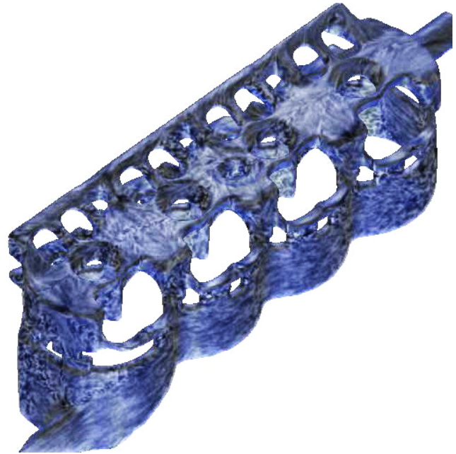
Figure 2: Visualization of flow at the complex surface of a cooling jacket -a composite of over 250,000 polygons.
