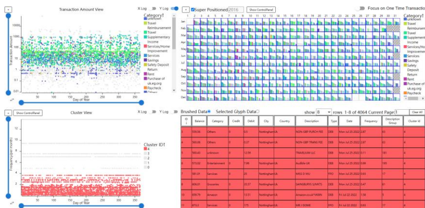
Figure 7.1.13.2. The cluster ID 4 is selected. As a result, the transaction amount view and the calendar view set the colour of the visual elements for the transactions whose cluster-ID is not four as grey. The table view only shows the data whose cluster-ID is 4.
