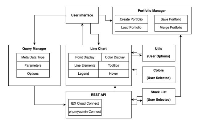
Figure 23: A schematic display of the software systems displaying the key subsystems and how they interact with each other.
