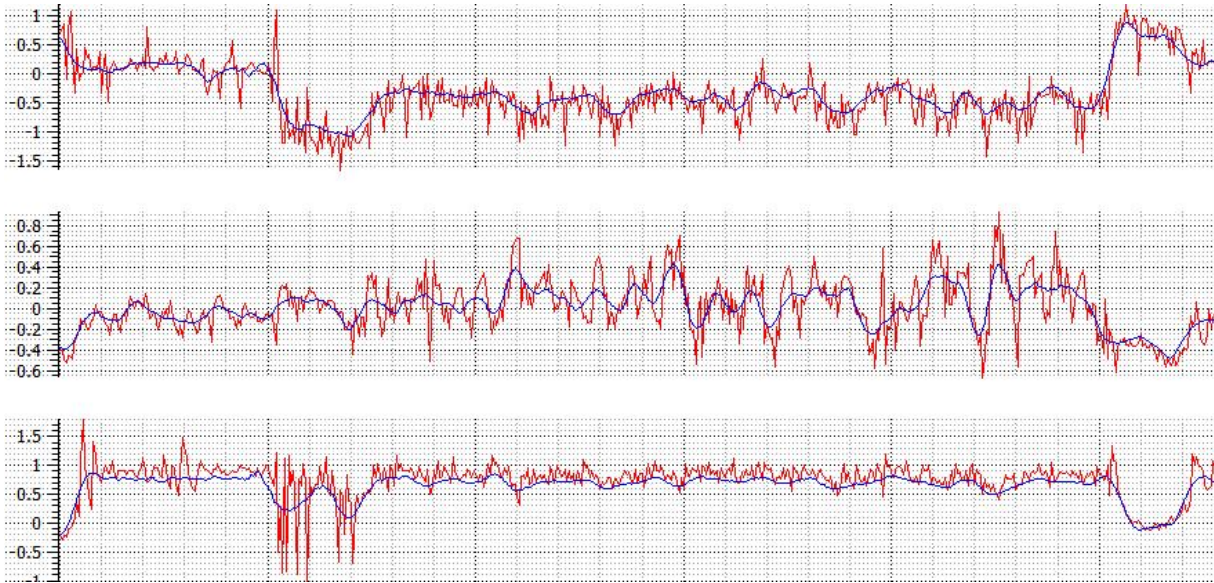
Figure 33: Stacked graph displaying tri-axel accelerometer data. The red curve displays total acceleration and the blue curve displays static acceleration derived using the Savitzky-Golay filter.
