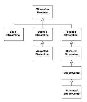
Figure 3: This is an example of a class hierarchy diagram. This example is from a class hierarchy of streamline and geometric flow visualization options. UML notation is used.
