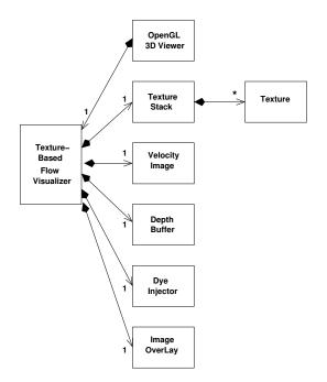
Figure 4: This is an example of a composition diagram. For example, the major components of the texture-based flow visualization design. Here aggregation, or *is-part-of*, relationships are shown.
