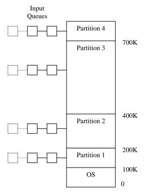
The diagram above shows how this scheme might work. The memory is divided into four partitions (we'll ignore the operating system). When a job arrives it is placed in the input queue for the smallest partition that will accommodate it.
