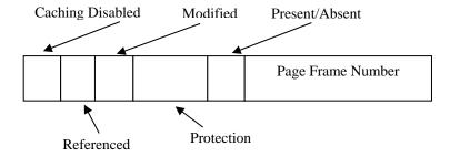
This diagram shows typical entries in a page table (although the exact entries are operating system dependent). The various components are described below.
