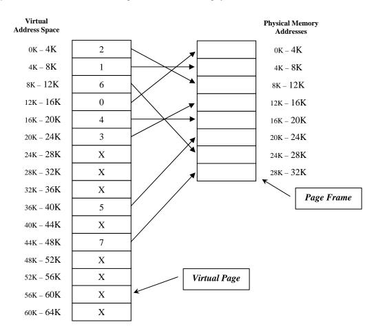
This diagram shows how virtual memory operates. The computer in this example can generate 16-bit addresses. That is addresses between 0 and 64K. The problem is the computer only has 32K of physical memory so although we can write programs that can access 64K of memory, we do not have the physical memory to support that.
