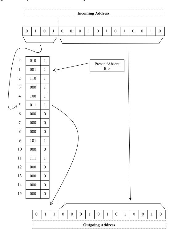
The incoming address (20818) consists of 16 bits. The top four bits are masked off and make an entry into the virtual page table (in this case it provides an index to entry 5 (101 in binary) and finds that this page is
