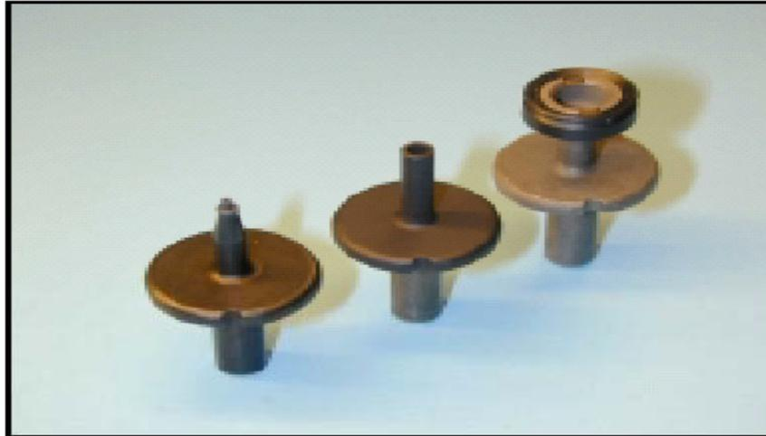
Figure 3.2: Example of vacuum nozzles.
