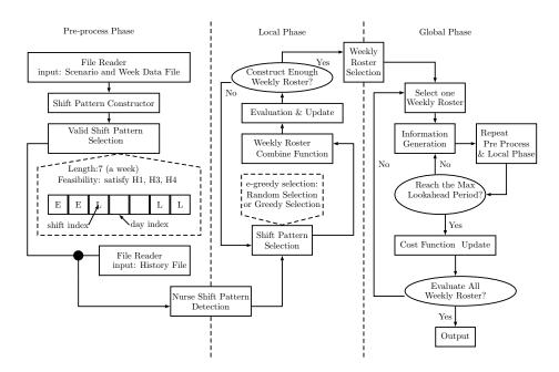
Fig. 1. Overview of the proposed algorithm applying ADP wit combined policy functions
