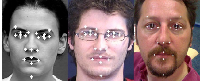
Figure 3. First-effort results of the utilized face point detector obtained for samples from (left to right): the Cohn-Kanade database, the MMI database, and a cell phone camera.
