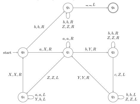
The formal definition of this Turing Machine is  $M = (Q, \Sigma, \Gamma, \delta, q_0, B, F)$  with set of states  $Q = \{q_0, \ldots, q_6\}$ , alphabet  $\Sigma = \{a, b, c\}$ , tape symbols  $\Gamma = \{a, b, c, X, Y, Z, \bot\}$ , initial state  $q_0$ , blank symbol  $\bot$ , and set of final states  $F = \{q_6\}$ .
