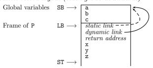
SB is Stack Base, LB is Local Base (or Frame Pointer), ST is Stack Top. The activation record (or frame) of the currently active procedure/function is the one between LB and ST. The solid arrow from the current activation record represents the dynamic link, i.e. it refers to the activation record of the caller and is thus
