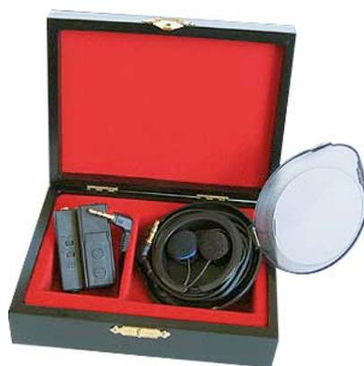
Figure 4 – In ear microphones. These look similar to normal in-ear ‘bud’ style headphones, but provide outward facing microphones. An internal audio pass-through means they do not serve as a barrier to normal hearing.
