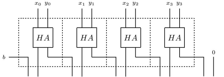
The component  $HA(x, y) = ((x + y) \bmod 2), (x + y) \text{ div } 2$ ) above is usually called a *half-adder*. If a large number of binary additions are to be done (such as in a multiplier circuit), a considerable speed-up can be obtained by first converting to carry-save numbers, and then doing all the additions using carry-save adders. Using this technique, the carry propagation which occurs when the final carry-save number is converted back to binary is amortized over many additions.
