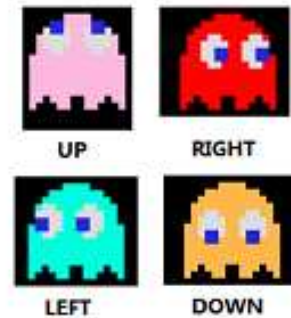
Fig. 3. These images show how the ghosts look in direction of travel so that we are able to determine the direction of a ghost by examining the pixels of the iris.
