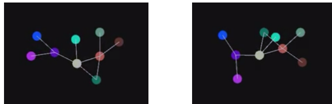
Fig. 1. Two runs of the same graph layout algorithm in which nodes repel each other, unless directly connected, in which case they also attract. Even with identical initial conditions, two executions converge to different stable configurations, demonstrating that pure FRP systems exhibit non-determinism.
