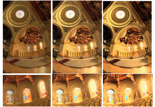
Figure 4. Top row: left to right, images mapped by the optimization method with \lambda = 0.5 , method of Ward et al [14] and histogram equalization. bottom row: amplified regions of the images above them. Radiance map dynamic range 340,016:1. Radiance map courtesy of Paul Debevec.
