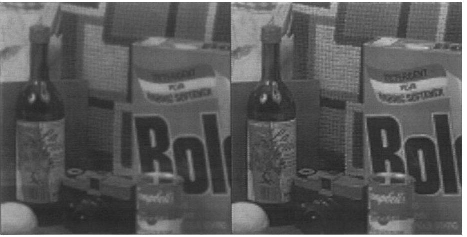
FIG. 9. Detergent image reduced and then expanded by a factor of 4 ( 512 \times 512 to 128 \times 128 and 128 \times 128 to 512 \times 512 ). Left: Bilinear interpolation. Right: Image improved by new method.
