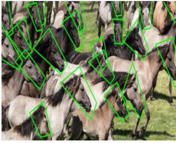
Figure 2: Mock-up of HABIT system interface, identifying and tracking individual horses in a herd
