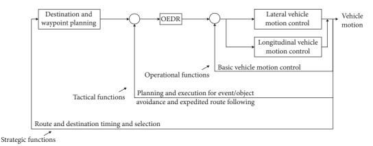
FIGURE 1: Schematic view of driving tasks [20].
