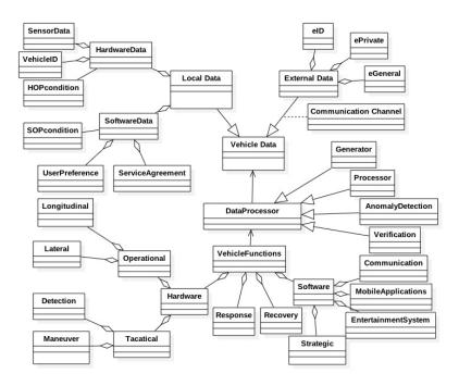
Figure 2. Unified Modelling Language (UML)-based CAV framework.
