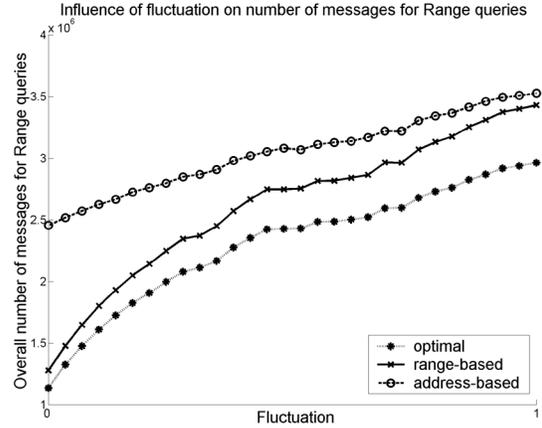
**Figure 7. Messages generated for Range queries against different fluctuation values**
