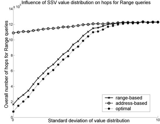
**Figure 5. Hops traversed for Range queries, against different degrees of value concentration**
