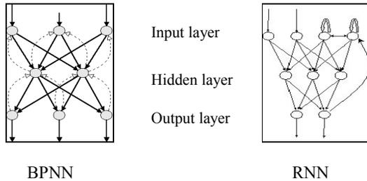
Figure 3 Architecture of BPNN and RNN
