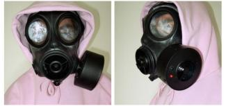
Figure 10. Respiration sensing, Wi-Fi enabled gas mask
