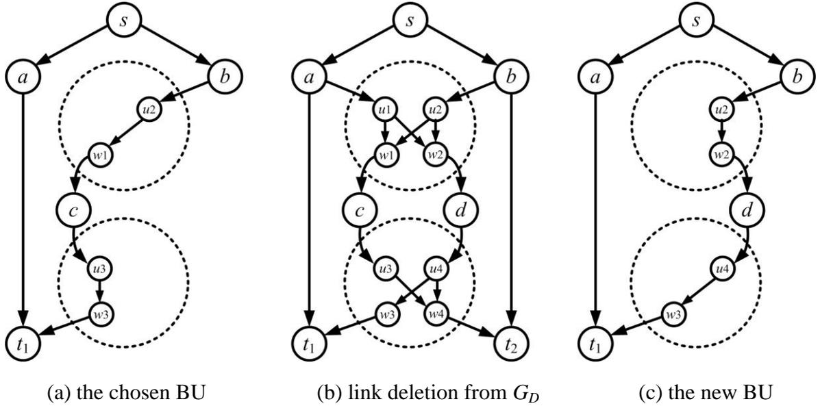
Fig.6 An example of the mutation operator  $M_1$
